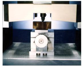
You can obtain in-situ indentation load-depth curve during indentation test. Through the software program loaded in the notebook computer, mechanical properties such as flow curve, yield strength, tensile strength and hardness can be estimated simultaneously. In addition, changes in mechanical properties such as weldment/HAZ/base metal and local material degradation can be analyzed immediately by the superposition of the obtained curves.
