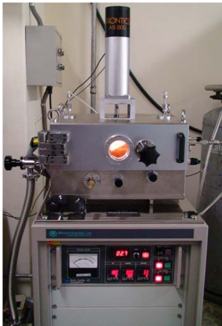
Fig. 2. High-temperature chamber system with IIT equipment.
