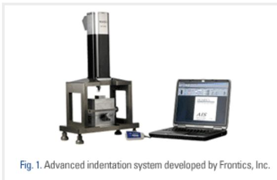
Fig. 1. Advanced indentation system developed by Frontics, Inc.
