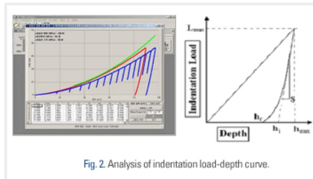
Fig. 2. Analysis of indentation load-depth curve.
