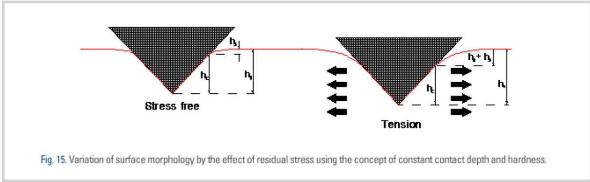
We have superimposed the common curve of contact load curve and indentation load curve at stress free situation and tensile stress situation
