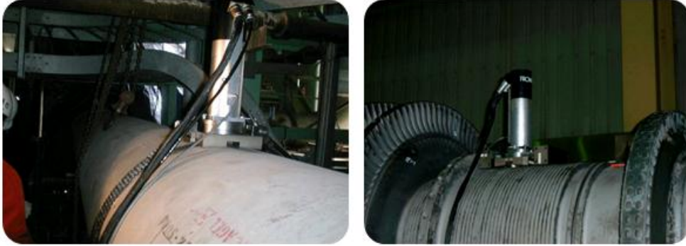
그림 18. Application cases steam pipeline and turbine at power plant inspection using non-destructive indentation technique (with KEPRI in Korea)
